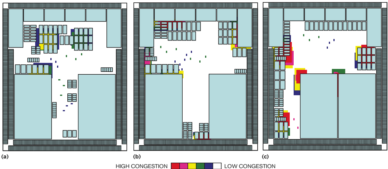
Figure 1 The congestion maps for three scripted-prototyping runs show a good implementation strategy (a), a slightly worse one (b), and a poor one (c).
